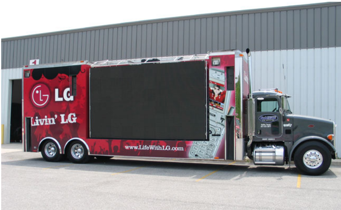
Figure 10. A 40 ft trailer with an integral LED video screen measuring 9x16 ft. The screen shows full motion video while the truck is moving in traffic, and can be raised to a height of 25 ft for viewing while parked.
